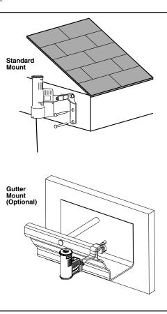
cause the Wireless Rain-Clik to dry out sooner than desired. Similarly, mounting on the northern end of a building with constant shade may keep the Wireless Rain-Clik from drying soon enough.
