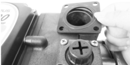
FIG 11 – PLACING GASKET ON FLANGE
