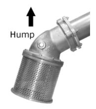
The flapper is not spring loaded which allows for a wide-open valve with very low friction loss. The valve requires a small amount of suction lift (vertical distance from the water surface to the pump center line) 4 feet is sufficient static head pressure to seal the valve.
