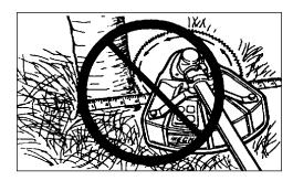
Use Shoulder/Waist Harness Use of the Shoulder/Waist Harness is recommended for ALL Trimmer/Brush Cutter use, not just Blade operation. The Shoulder/Waist Harness when used in a trimming operation with nylon line head suspends the trimmer from the operator's shoulder and reduces operator fatigue.
