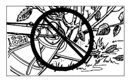
8 Tooth Grass and Weed Blade is designed for grass, garden debris and thick weeds up to 19 mm (3/4") diameter. DO NOT use this blade for brush or heavy woody growth.
