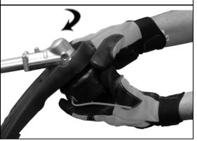
Hold trimmer head while turning knob clockwise to wind line onto spool until about 5" (13 cm) of each line remains exposed.
