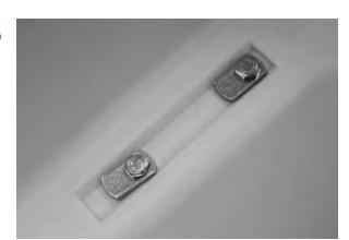
Put the hole in the washer over the front (larger) hole. Rotate the washer so the long, flat area covers the second hole. Repeat for all four holes, then put the bolts through and tighten.
