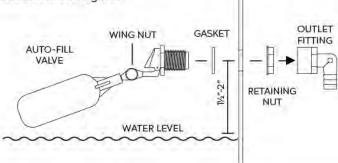
The Auto Fill Kit includes fittings for connection to a garden hose, ½" irrigation line, and ½" Sch 40 PVC. Wrap the ½" male threads on the Auto Fill with thread sealant and install the fitting of your choice. Once water is supplied to the Auto Fill it will maintain the set water level by automatically adding water when the level drops. This level can be adjusted by loosening the wing nut and raising and lowering the height of the Auto Fill float.
