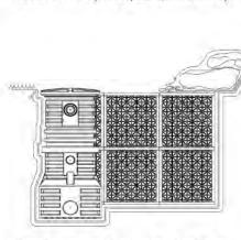
Once excavation is complete, install underlayment, pond liner, properly oriented Eco-Blox and Pump Vault. Backfill the space between the Eco-Blox/ Pump Vault and the excavation to lock them into place, either outside the liner with sand or clean fill, or inside the liner with gravel \(^3\)\" or larger in diameter. Top the liner and basin with \(^3\)\" or larger gravel or decorative stone.
