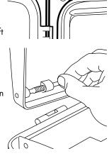
the panel hinge pin at the top drops out of the retaining hole in the housing. Set the control panel door aside in a safe place. Note: The SLCP control panel does not need to be removed from the control panel door during Installation.
