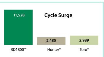
This comparison test also shows average cycles to failure for competitive 4" spray head models including check valves and 30 psi pressure regulation. Each cycle consists of 3 seconds on at 200 psi and 2 seconds off. Tested to failure is defined as damage or non-correctable leaks. Tests conducted at Rain Bird Product Research Center in Tucson, AZ.
