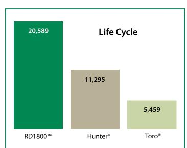
This comparison test shows average cycles to failure for competitive 4" spray head models including check valves and 30 psi pressure regulation. Each cycle consists of 30 seconds on at 100 psi and 30 seconds off. Tested to failure is defined as damage or non-correctable leaks. Tests conducted at Rain Bird Product Research Center in Tucson, AZ.
