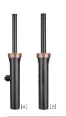
[A] PROS-06-SI-PRS30 [B] **PROS-06-PRS30** Retracted height: 83/4" Pop-up height: 6" Exposed diameter: 21/4" Inlet size: 1/2"
