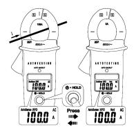
Data Hold is not available when "OL K $\Omega$ " is displayed with no input signals.
