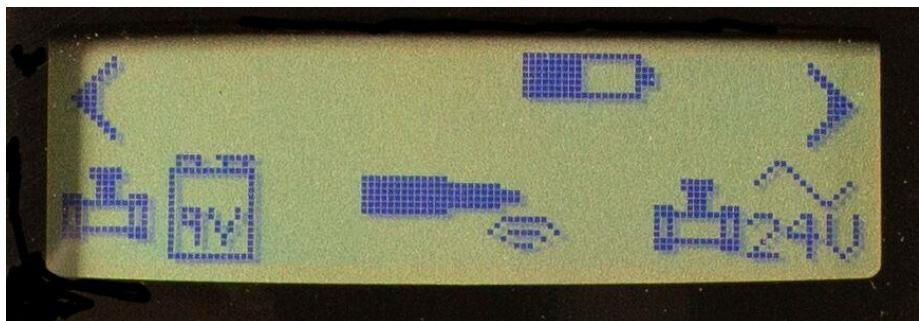
**F1: Operation with battery-powered controllers and remote DC latching valve solenoids.**
