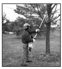
Look out for the branch immediately behind the one being cut. If the saw chain hits the rear branch damage to the saw chain may occur (or kickback).
