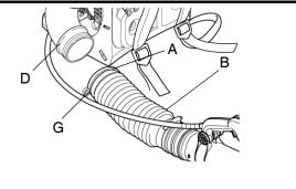
5. Assemble flexible pipe (B) to elbow (D) on blower. Position guide loop (G) on outside of flexible pipe (away from blower) and tighten clamp (A).
