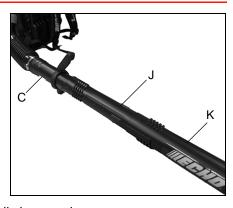
Note: Blower use will eventually loosen pipe connections. Exclusive positive locking system allows pipes to be tightened. If loosening occurs, remove two straight pipes and install according to instructions 8 & 9
