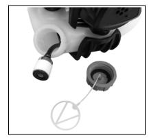
Do not damage fuel line while removing fuel filter from tank.
