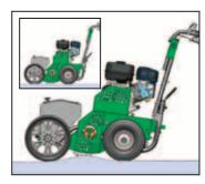
Floating cutting head with an exclusively designed 22" (56 cm) slicing reel floats with contours of yards, increasing seed to soil contact & improving germination rates.
