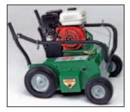
Fold-n-Go™ no tool, no bolt foldable handle with inside bail and padded handles. Great for comfort, storage, transport and long life. (PR550 unit shown).
