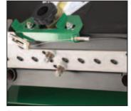
Auto Drop™ system automatically starts and stops seed drop with reel engagement & disengagement, conserving valuable seed. Spring loaded stainless steel slide prevents binding if clogging occurs and is easy to clean. Spring loaded hardware eliminates corrosion.
