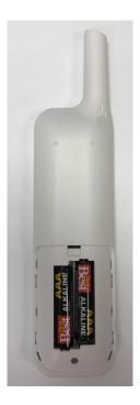
Replace cover by snapping the cover back on the unit.
