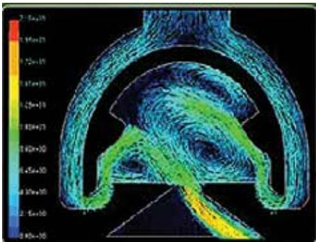
Water expands and collapses inside the H<sup>2</sup>O Chip created high-frequency oscillating streams which allow for distance of throw using 1/3 less flow.
