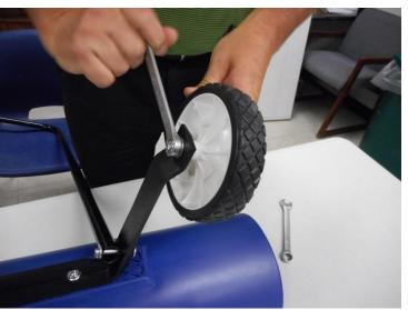
Tighten nuts using the 9/16" wrench and the adjustable wrench to hold both the bolt head and nut during the tightening process. The self-locking nut will require more force to tighten than a standard nut.
