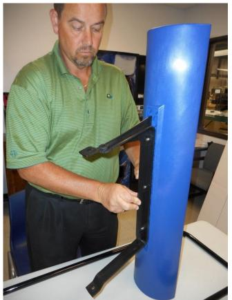
Insert three (3) - 1" X 5/16" carriage bolts through face of blade into holes in the mating bracket. Be sure to align the square portion of the bolt head with the square opening in the face of the blade.
