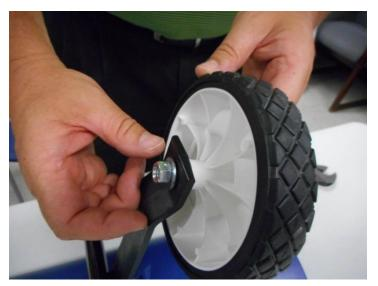
Install the wheel into the bracket by inserting the clevis pin through the bracket. Install one (1) - 5/16" washer on the clevis pin. Install one (1)- 3/8" self-locking nut by hand. Hand tighten the nut.
