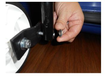
Start threading each of the (3) - 5/16" self-locking nuts by hand.
