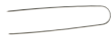
6" Soil Staple (Place approximately every 3'-5' of tubing, plus two on each tee, elbow or cross) Model TLS6
