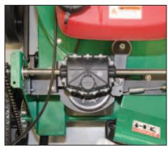
**Single speed rear self-propelled** is great in hilly turf applications. (KV601SP, KV650SPH and TKV650SPH only)
