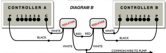
STEP 1: CONNECT BLACK / WHITE PAIR OF WIRES TO THE CONTROLLER.
