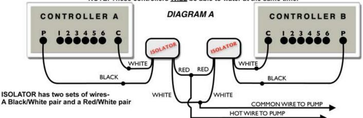
STEP 1: CONNECT BLACK / WHITE PAIR OF WIRES TO THE CONTROLLER.
