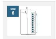
Connect field and common wiring as needed and test.
