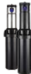
I-20-04 Overall height: 7½" Pop-up height: 4" Exposed diameter: 1¾" Inlet size: ¾"
