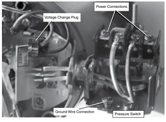
Figure 4: Voltage set to 230 volts, Plug Type
