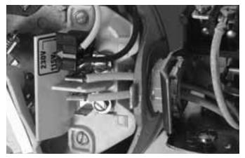
Figure 5: Voltage set to 115 volts, Plug Type
