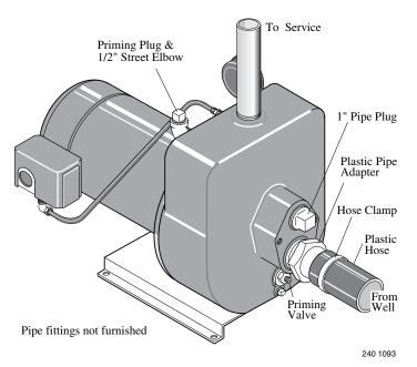
Figure 3 - Shallow Well Installation
