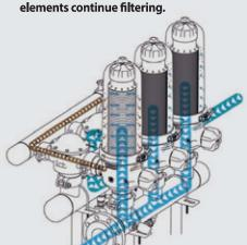
**FILTRATION STAGE:** As water goes through the discs, particles are projected away due to the cyclone effect, reducing the backflushing frequency.
