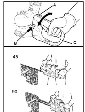
4. Grip the throttle handle. Press the throttle lockout lever down with palm of hand and squeeze throttle trigger (D) to reset rotation release button (B), and lock handle in position.
