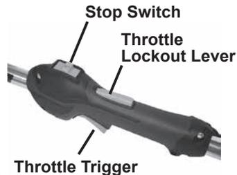
**NEVER** fuel, start, or operate your unit unless it is fully assembled, all shields and required guards are in place, and the throttle lock-out lever and trigger are working properly.
