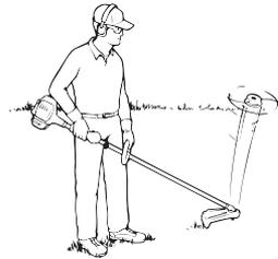
**Make sure line head is securely fastened**
