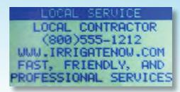
The **Contractor Message Screen** allows the contractor to input a custom message with their name and contact information into the controller from the software via a USB drive so it is visible to the homeowner when they press the "Help" button.
