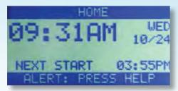
The **Home Screen** displays the current time and date, what zones are scheduled to water next, or if currently watering, what zone(s) are currently watering and how much time is remaining, as well as any alerts – in the absence of any alerts, the screen will display "SYSTEM OK."
