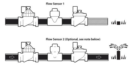
To measure flow from 2 water sources a device that scales the signals from two flow sensors and combines them into one digital output is needed. Use Combiflow CBF-100-00 or equivalent.
