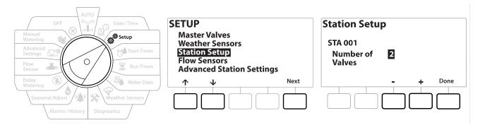
Setting the number of valves to 2 will not control them individually, it will only adjust the output voltage to ensure both valves open.
