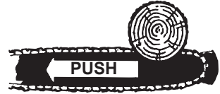
CUTTING ON TOP OF GUIDE BAR PUSHES SAW TOWARD YOU
