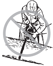
KEEP BODY OUT OF CUTTING PLANE
