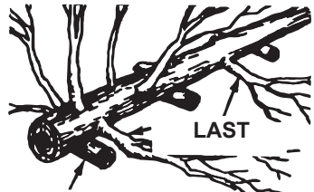
USE SUPPORT LOG UNDER TRUNK - LEAVE SUPPORT LIMBS UNTIL LAST
