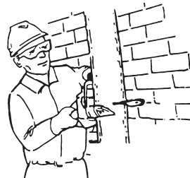
KICK GUARD ALLOWS KICKBACK FREE CUTTING NEAR MASONRY, FENCES, ETC.
