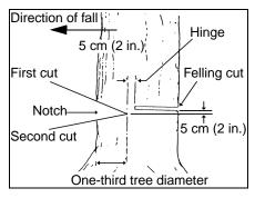
guiding it in the desired direction. When the tree starts to fall, kill the engine, place the saw on the ground and make your retreat quickly.
