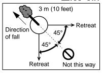
Begin the cut on the side to which the tree is to fall. Cut a notch about 1/3 of the way into the tree. The position of this notch is important since the tree will try to fall "into" the notch. The felling cut is made on the side opposite the notch and at a level about 5 cm (2 in.) above the bottom of the notch. Do not try to cut through to the notch with the felling cut. The remaining wood between the notch cut and felling cut about 5 cm (2 in.) will act as a hinge when the tree falls,
