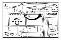
Do not turn the adjusting screw beyond the maximum or minimum limit of volume adjustment.
