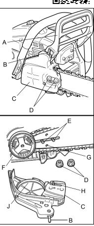
Install sprocket guard over guide bar studs. Ensure chain tension adjuster pin (H) fits into the guide bar adjuster hole (G), brake band (J) is positioned around clutch drum. Tighten sprocket guard nuts finger tight.
