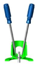
Figure 15 - Remove Mechanical Seal
