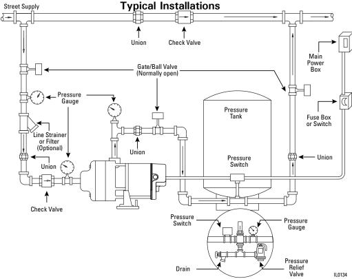
To size pressure tank properly, match the drawdown of the tank to the capacity of the pump.
