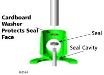
Figure 17- If Necessary, Press with Cardboard and Pipe
