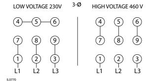
Figure 9 - Wiring Diagram for Three Phase
