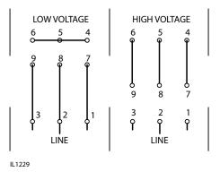
Figure 10 - Wiring Diagram for Baldor TEFC 3 Phase motors
