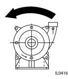
Figure 14 - Correct Motor Rotation
