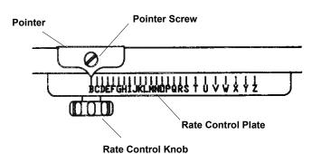
2. Flip on/off control lever to the "ON" position. Check the port opening. It should be just open. If adjustment is necessary, continue to step #3. **3.** Loosen the rate control knob and slide the rate plate until the port is just opening. Loosen pointer screw and move pointer until it aligns with "B" on the rate plate. Retighten pointer screw.
