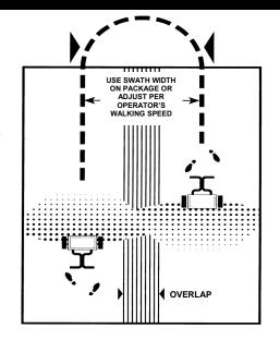
**6.** Push spreader at a normal walking speed -2 1/2 m.p.h. (18 feet in 5 seconds). Apply header strips around area to be treated. Space trips across the area as shown. Keep material off flower beds, sidewalks, etc.
