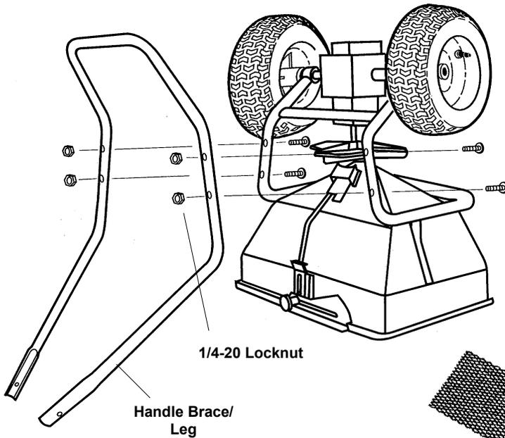
**3. Turn spreader upright on wheels. Insert screen into hopper sliding it under the screen clips. Attach the upper handle assembly to handle brace with the handle lever facing as shown. Secure with (2) 1/4-20 x 1 1/2" carriage bolts, and locknuts.**
