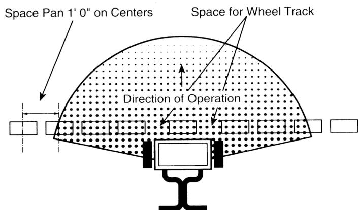
Once the pattern is uniform, the effective pattern width can be determined. The effective pattern width is the distance out from the spreader to a point where the amount of material is 1/2 the average amount in the center pans. This distance is multiplied by 2 to achieve the total effective pattern width.
