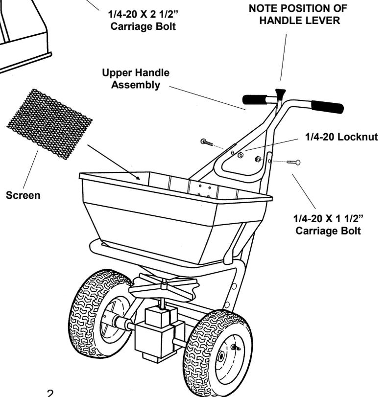
**4.** Install control tube to handle lever with (1) 1/4 dia. clevis pin and a 3/32" dia. cotter pin. Slip opposite end of control tube over lower control rod making sure shutoff plate is between the lower rod and the control tube. Secure with a 3/32" dia. hitch pin cotter.
