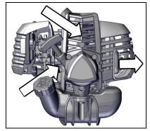
Dust and grass build up on the outside of the cylinder. This build up insulates the engine and prevents the heat from leaving.
