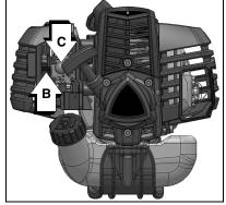
grasp throttle handle and throttle trigger lockout with left hand and fully depress throttle trigger to wide open position. Rapidly pull recoil starter handle/rope (D) until engine fires (or maximum five [5] pulls).
