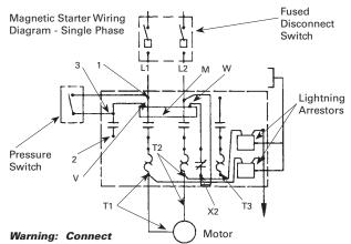
Warning: Connec motor leads momentarily for correct rotation Figure 5
