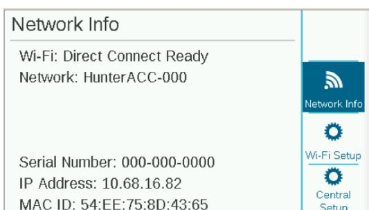
Use the dial to go to Settings, Networking. Verify the address of the controller by viewing Network Info screen. Press soft key for Wi-Fi Setup. Check the box for Direct Connect. (The Central Setup function is not currently active.) Open mobile device settings for Wi-Fi and search for HunterACC-xxxx (where -xxxx is the unique four digit number shown at Network Info), and connect.
