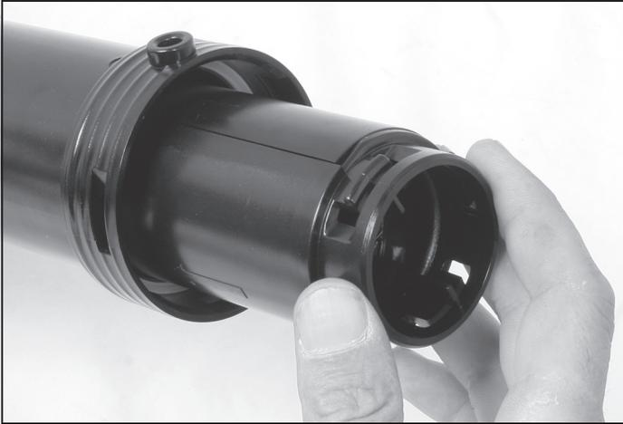
3. With the sleeve fully removed it can either be cleaned or replaced.
