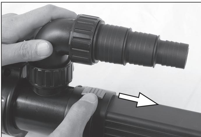
3. Rotate the ballast counter-clockwise about ½" to release it from the locked position and carefully slide out the ballast with quartz sleeve attached.
