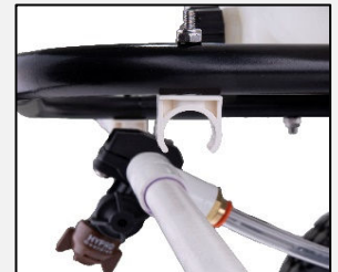
Boom clips allow easy change between the applicator booms.
