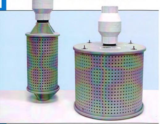
Big Foot Filters are designed to be used as an initial filter on the suction side of a pump using surface water sources. The 40G and 80G, rated at 40 gallons per minute and 80 gallons per minute respectively, are made of heavy duty PVC plastic. Extra large intake areas will require little or no service during the pumping season and will give many years of trouble free service, even under the most severe conditions.
