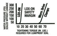
Performance graph shows sealing results of all stainless Lox-On compared to average of four brands of all stainless worm drive clamps on 1" polyethylene pipe over a 0.985" smooth plug.
