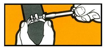
Bend band at  $90^{\circ}$  from buckle and engage outer tooth with serration. Hold band down and tighten screw.
