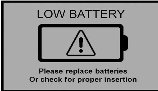
In addition to frequency of use, battery life is impacted by use of the backlight and GPS receiver. If not needed, the GPS feature should be disabled. The backlight can be set to AUTO mode (p. 12). This allows enough time to see the reading without unduly taxing the battery.
