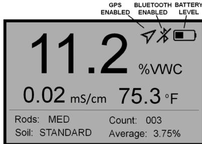
When disabled, the GPS and/or Bluetooth icons will no longer be visible. When visible, the GPS icon will indicate the quality of the GPS fix (p. 27).
