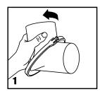
Rotate fitting to desired angle.
