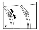
Lock angle in place by completely closing both locking ring clips
