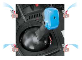
**QUICK STICK® CHUTE CONTROL** Innovative joystick control allows you to change chute direction and angle quickly and easily on the go.
