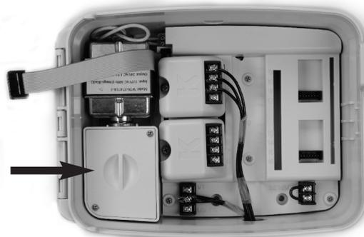
The Pro EX 2.0 controller is powered with either 115VAC or 220VAC which must be noted when ordering the unit.
