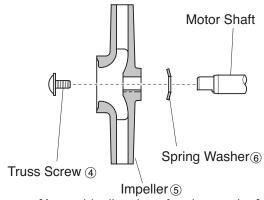
[Assembly direction of spring washer]
