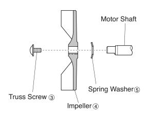
[Assembly direction of spring washer]
