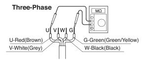
**Note:** The insulation resistance reference value of  $20M \Omega$  minimum is based on a new or repaired pump. For reference values of a pump that has already been put into operation, refer to "7. Maintenance and Inspection" of this manual.
