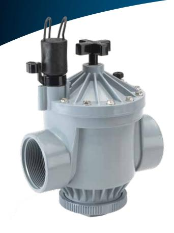
The Irritrol® 200B Series globe/angle valves have built their popularity on a proven record of reliability and a reputation for offering valuable features at an affordable price. The 200B Series provides manual internal and external bleed, heavy-duty, UV-resistant PVC construction, stainless steel hardware, a double-beaded diaphragm and a captive solenoid plunger.
